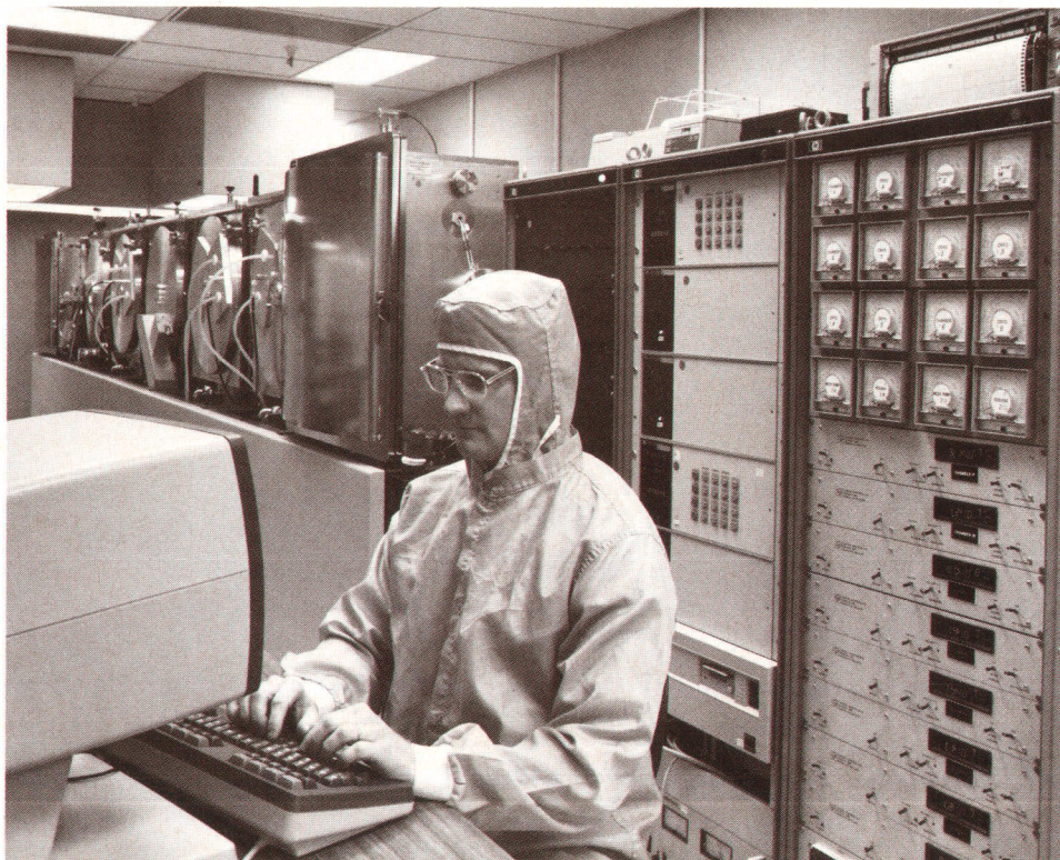
Fig. 1. In-line deposition system developed by HP for fabrication of thin-film magnetic discs.
